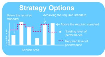
→ Reduce the level of performance: If the level of performance exceeds the required standard is unaffordable it should be reduced. For example, the frequency of maintenance might be reduced or the intervention level might be increased.
