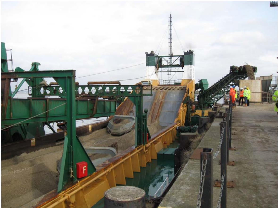
Figure 6 - Discharging marine dredged sand and gravel from a dredger
