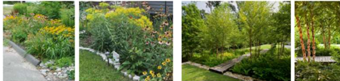
① Rain gardens - SuDS that capture rainfall before it enters the piped network and allows it to infiltrate into the ground.
